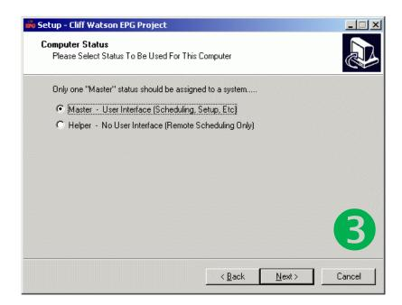
Select **Master** for the installation on the PC where you will be setting up CW\_EPG operations. Select **Helper** on any other PCs that you will be using with CW\_EPG for centrally controlled scheduling.
